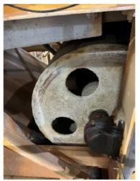
Perforated Drum with Heavy Material Build up
